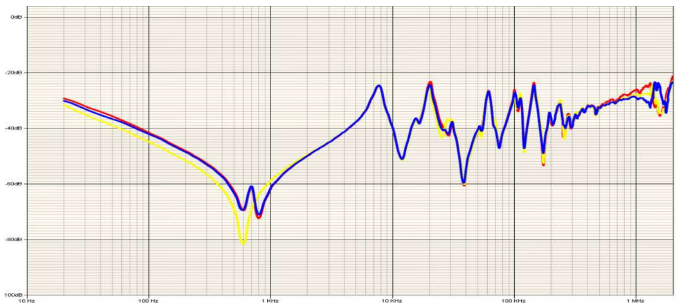
Sweep frequency response analysis trace
